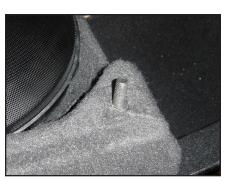
Thread the two included 3/8-16 x 2 1/4" Set Screws into the threaded inserts in the Stealthbox® leaving approximately 1/2" exposed.
